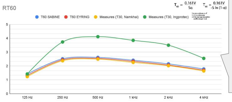
The curve resulting from the equations is regular with respect to the measurement, further fitting coefficients are applied.
