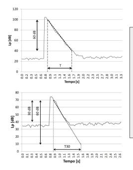
Ideally, you would like to measure the 60dB decay, but the low volume and the considerable sound power required do not allow this. You opt for the optimal T30 measurement version.
