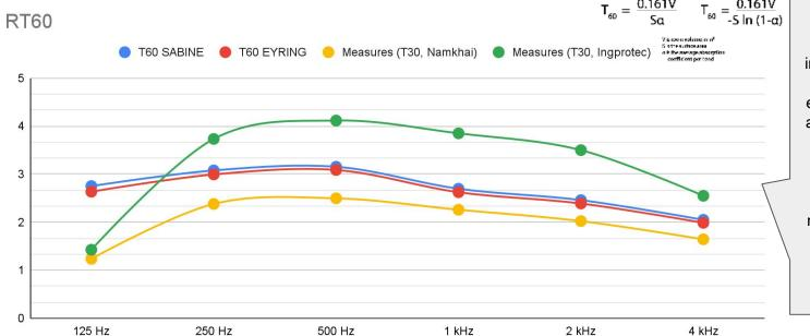
With the available information, a model is built based on the equations valid for low absorption coefficients in the diffuse field, obtaining a reverberation time similar to the one measured, also taking into account the air given the volume.
