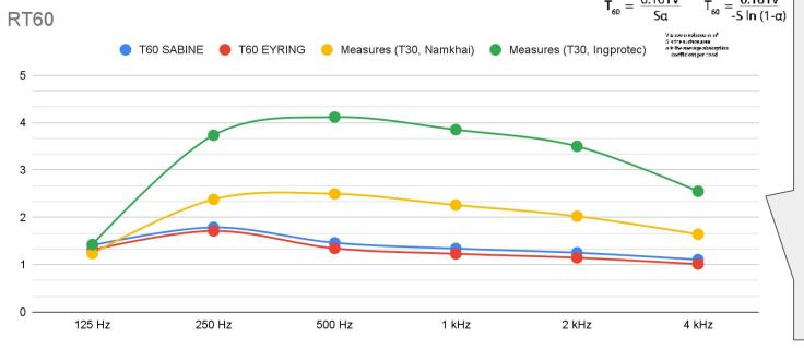
It considers 0.99 as the maximum sound absorption value, so the expected result will be better than the prediction especially for the most disturbing (low) frequencies.
